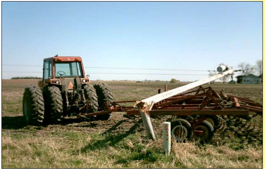
A primary line carrying 7,200 volts of electricity fell on this tractor when the driver came too close to the electrical pole.
