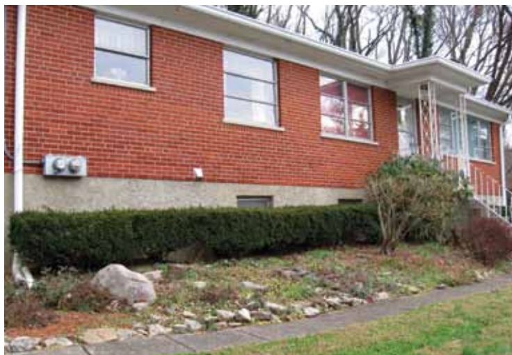
Dwarf shrubs block the wind, and the rocks capture the sun's heat during winter. During summer, trees shade the house wall and rocks.
