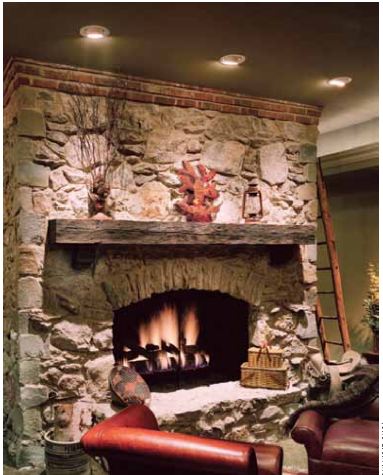
Adjustable eyeball recessed light fixtures are ideal to focus light on a specific object on the wall or floor.
