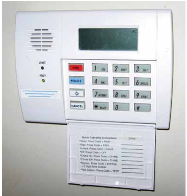
This wall-control module for a monitored security system boasts colored buttons for police, fire, and health emergencies.
